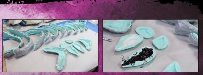
The 3D printed parts are to stiff and not very comfortable to wear. All parts were molded and then casted with a semi-rigid resin which makes it flexible.
