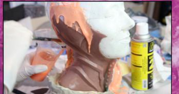
Brush-on Silicone is the best you can use to make simple and fast silicone molds. Brush on several layers until the mold is thick enough.
