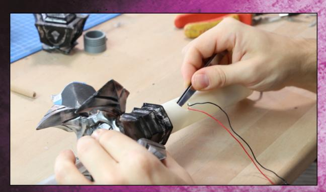
The electronics and the powerbank are hidden in the handle. The back of the handle can be screwed off to change the power bank.
