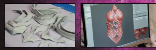
All parts for the breast plate were 3D modeled and printed.
