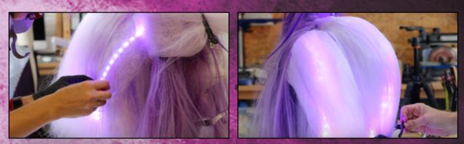
Add LEDs stripes to make the wig light-up. The fluffy hair is also perfect for diffusing the LEDs.
