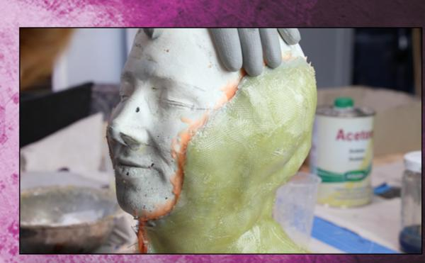
To keep the silicone mold in shape, you need a fiberglas jacket. It is made out of several layers epoxy resin and fiberglas matts.
