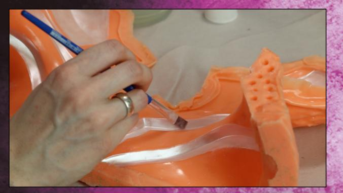
For the silver lines on the collar you can brush on metallic pigments directly into the silicone mold before adding the resin.
